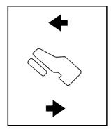
The switch used to adjust the pedals is located on the instrument panel below the climate control system. Press the arrow at the bottom of the switch to move the pedals closer to your body. Press the arrow at the top of the switch to move the pedals away from your body.
